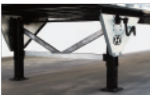
Steel bolt-on Wing Plate and bolt-on "K-bracing" between landing gear legs are Hot Dipped Galvanized
